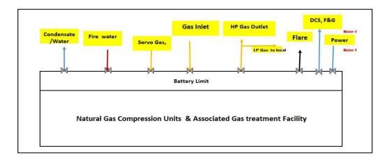
3.4 The scope of work involves design, engineering, procurement, fabrication, transportation, installation, hook up & commissioning of Sales Gas Compression and Gas Treatment Facility. The Compressors and Gas treatment units shall be skid based.
